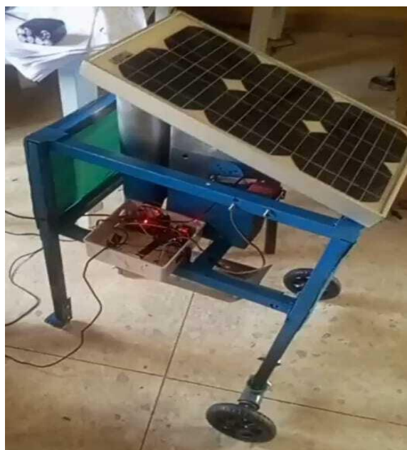
Figure 9; Fully assembled components of the Robotic Maize Seed Planter
